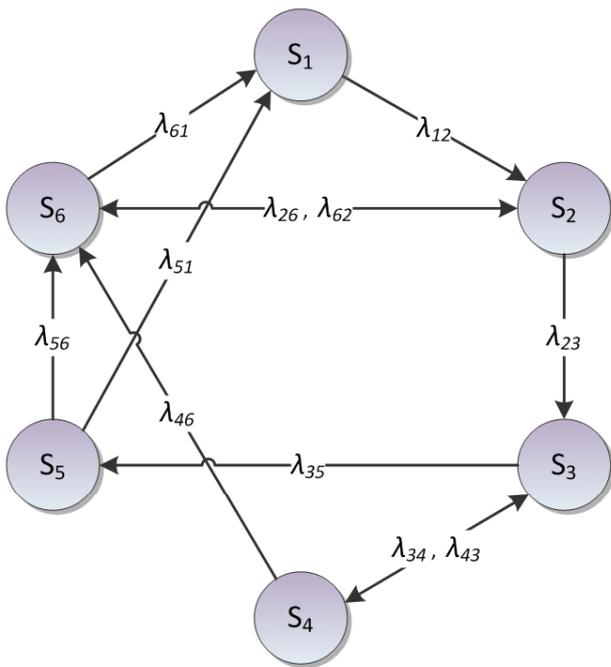
**Figure 1.** Directed graph of operating states of Diamond DA 20-C1 aircraft.
