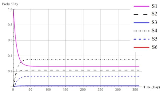
**Figure 2.** Probabilities of being in one of analysed operating states as a function of time, assuming that the initial state was the standby state for Diamond DA 20-C1.
