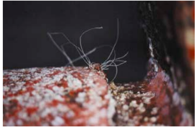
Figure 7. Nylon fishing line of a fishing net line screwed into the stern tube seal
