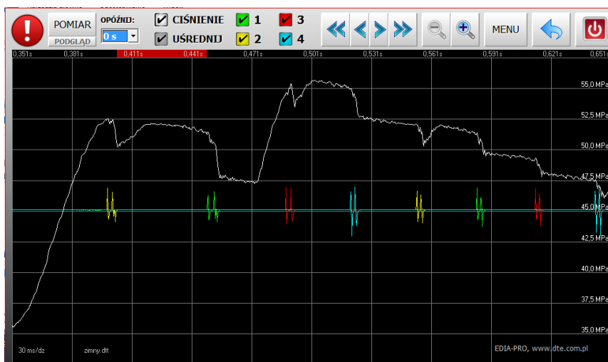
Fig. 4. Analysis of signal trajectory in the temporal analysis mode for uneven engine operation
