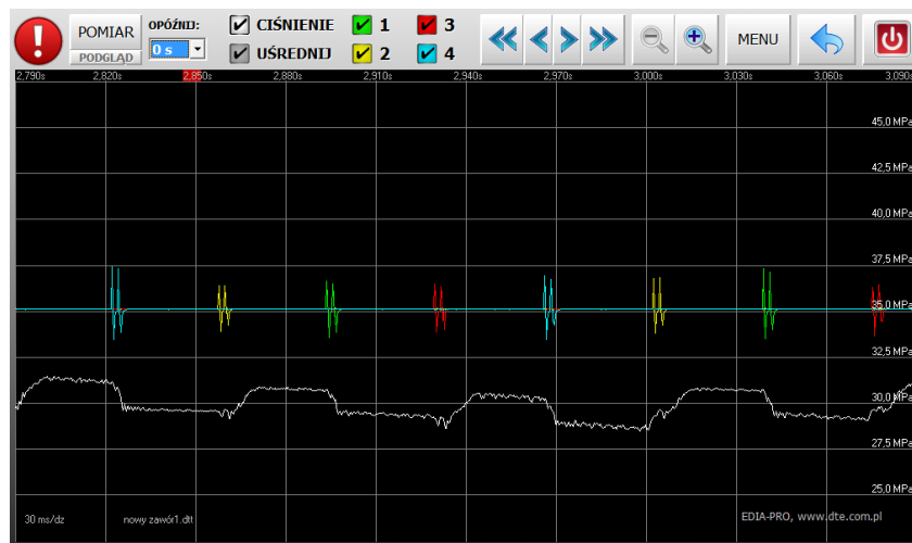
Fig 5. Analysis of a signal trajectory in the temporal analysis mode for even engine operation
