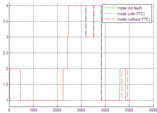
Fig. 27. Evolution of modes in: no fault case, Diagnosis case, FTC case
