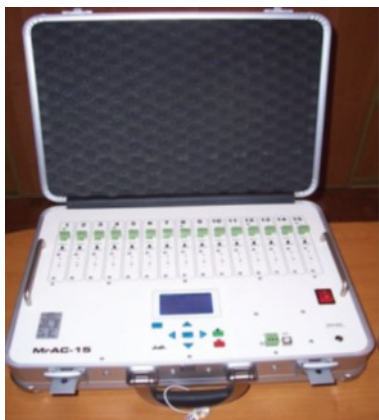
Fig. 3. View of an MrAC-15 multi-channel recorder
