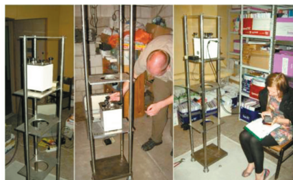
Fig. 20. The stand constructed by WUT (left) and IGK (right) for vertical gravity gradient determination at field station and laboratory station, respectively
