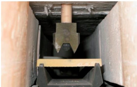
Fig. 4. The four-point strength measurement
