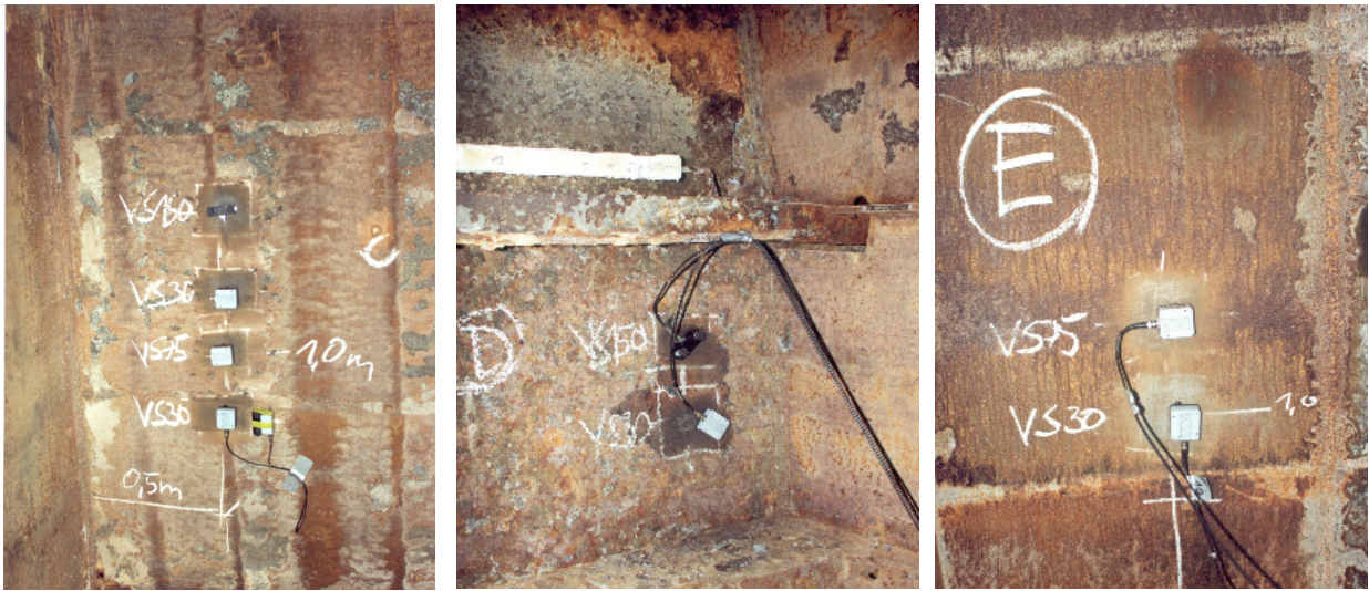
Fig.11 Marked and cleaned areas for fitting sensors at "C" measurement point and marking of sensor types and numbers on the surface of a wing tank bulkhead
