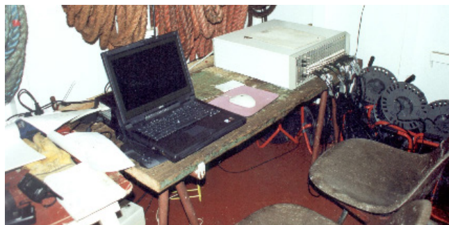
Fig. 12 16-channel measurement system and a docking station with a laptop in a bow room.
