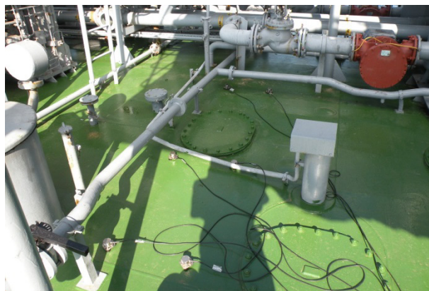
Fig. 16 Cargo deck of ORP Bałtyk'with sensors arranged for tests.
