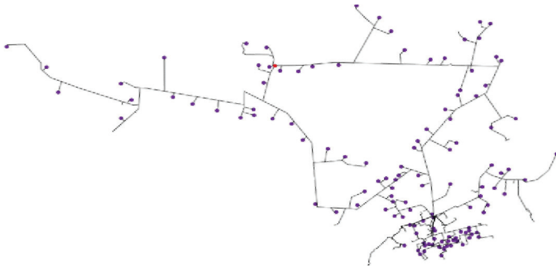
Fig. 3. KSN grid supplied from GPZ1, purple dots – MV/LV transformers – not included in the calculation
