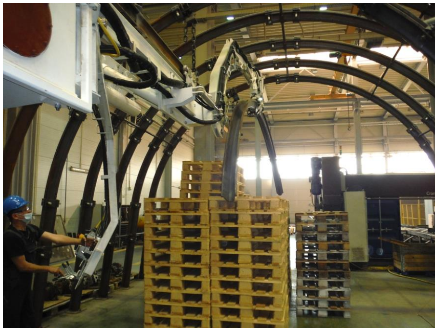
Fig. 7 Ride of the manipulator loaded with the support arch over the roadheader and the operator's cabin (pallet) with the stabilizing foot folded
