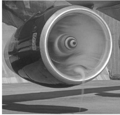
Fig. 1. Operation of turbojet engine inlet RB211-524G by Rolls-Royce on the ground (pic. P. Thomas)
