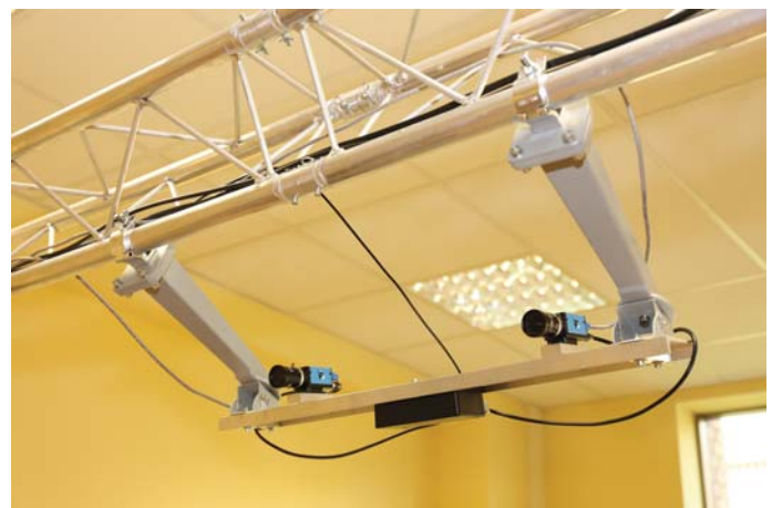
Fig. 1. Wide field of view vision system
