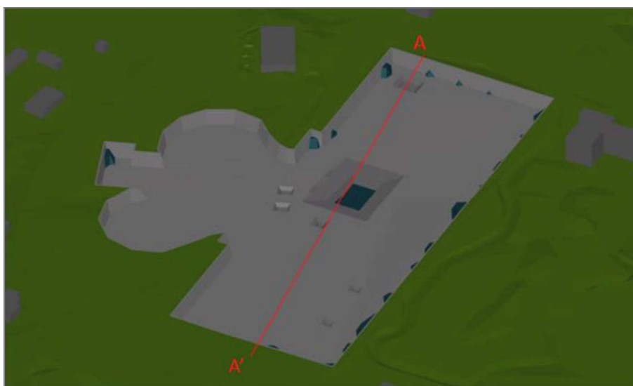
Fig. 15. Visualization of groundwater surface with reference to DSM (digital slab model), Stage VIII
