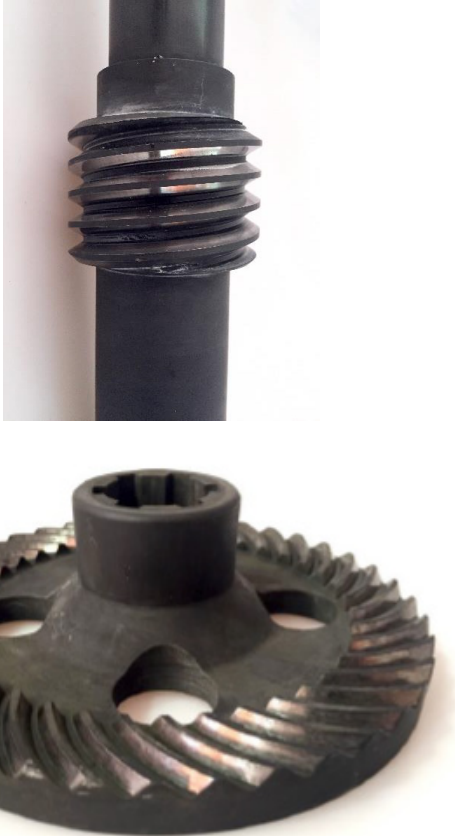
Figure 3. Both elements of spiroid gears: worm thread and face gear in real.
