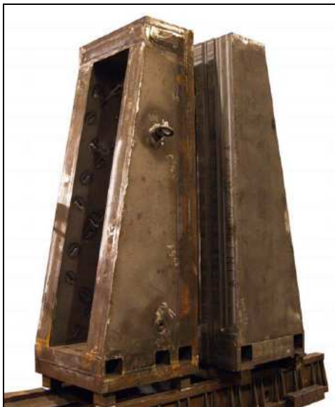
Fig. 16. One of the experimental arrangements of both columns (common and alternative) for static stiffness measurement
