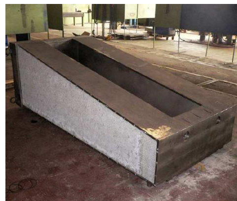
Fig. 15. Alternative column with glued-on cores before montage of side covering plates.
