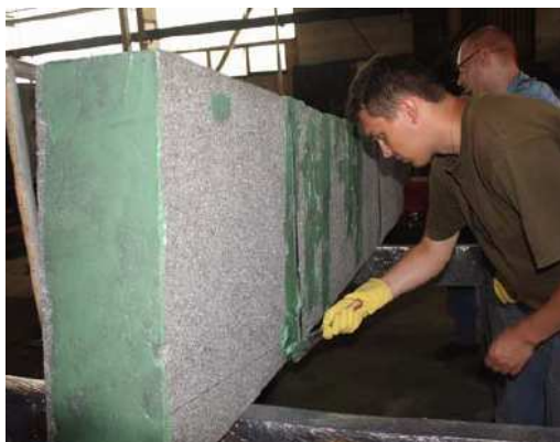
Fig. 14. Alternative column manufacturing. Picture shows glue application on the aluminium foam core (made from Alporas foam)
