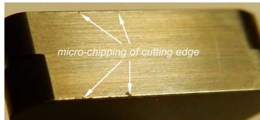
Fig. 5. Characteristic cutting edge micro-chipping of CBN inserts
