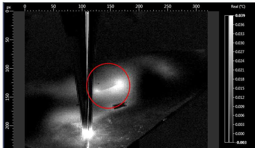
Fig. 3. Specimen after excitation. There is possible to see crack with I shape
