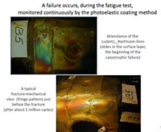
Fig. 5. Photoelastic visualisation of fatigue test.
