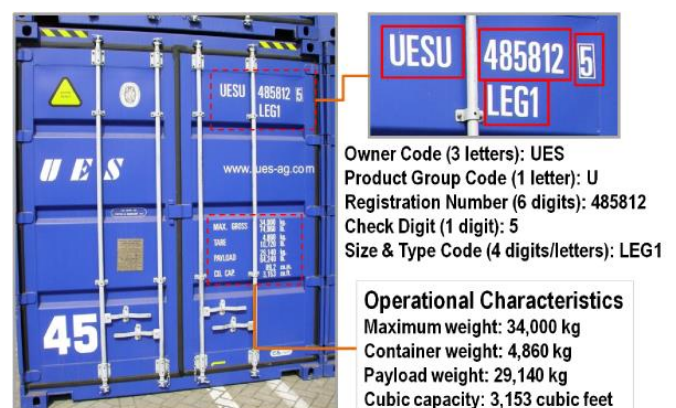
Fig. 2. Sample of container labeling [6]
