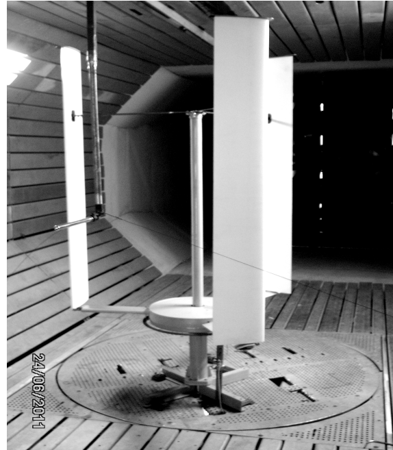
Fig. 1. The wind rotor with controlled blades in the wind tunnel
