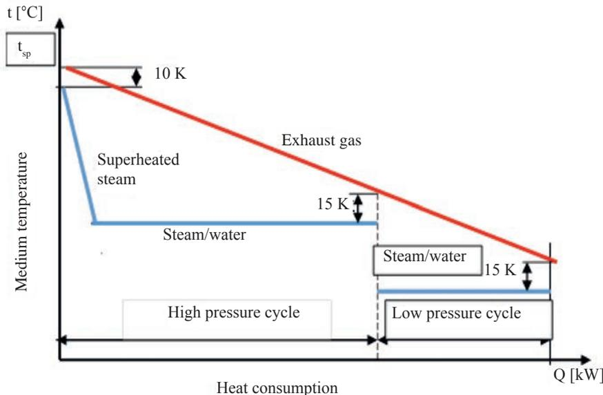
**Fig. 4. Distribution of temperatures in the double-pressure waste heat system**
