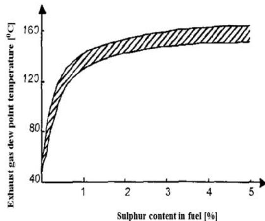
**Fig. 2. Impact of sulphur content in fuel on exhaust gas dew point temperature**
