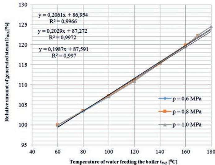
**Fig. 1. Impact of temperature of feeding water and working pressure on the amount of steam generated in the waste heat recovery boiler**
