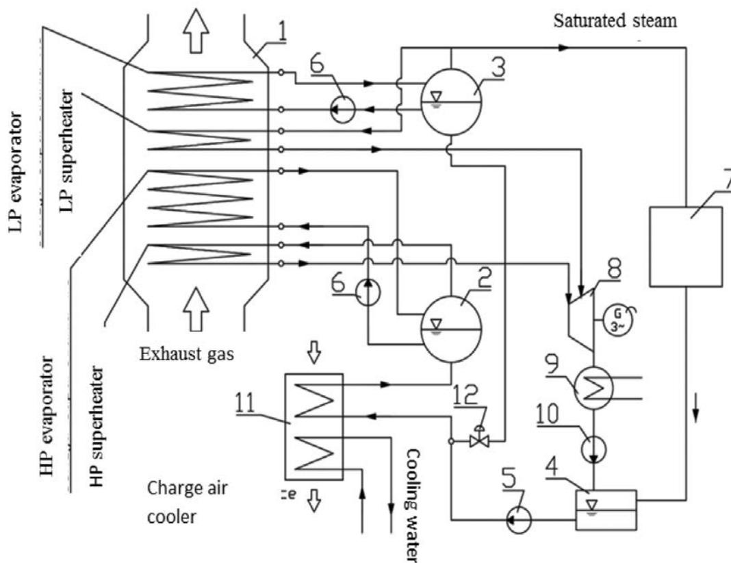
Fig. 3. Waste heat recovery system based on the solution of MAN-B&W: 1 – waste heat recovery boiler, 2 – HP steam-water boiler drum WC, 3 – LP steam-water boiler drum, 4 – hot well, 5 – pump feeding boiler, 6 – circulation pump, 7 – heating steam receivers, 8 – turbogenerator, 9 – condenser, 10 – condensate pump, 11 – charge air cooler, 12 – pressure reducing valve, HP – high pressure, LP – low pressure
