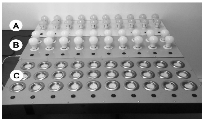
Fig. 4. The three additional panels (boards) with mounted LED lamps: A) E14 base, B) E27 base, C) GU10 base
