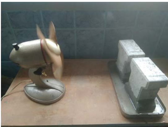
Fig. 4. . Efflorescence observation test of Zeol ICB
