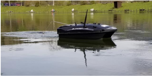
Photo 1. Radio-controlled aquatic drone used to transport the sonic sensor into the measured lakes (phot. R. Giusti)
