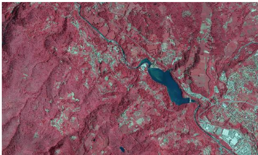
Fig. 2. Portion of orthophoto obtained with a near infrared sensor: Pontecosì dam on the Serchio River – Lucca province; data used: ‘Ortofoto 20 cm copyright 2016 Consorzio TeA’ OFC 2016 20 cm –32 bit colour – 4R 1G 2B NirRG Standard False Colour for vegetation studies; source: own elaboration
