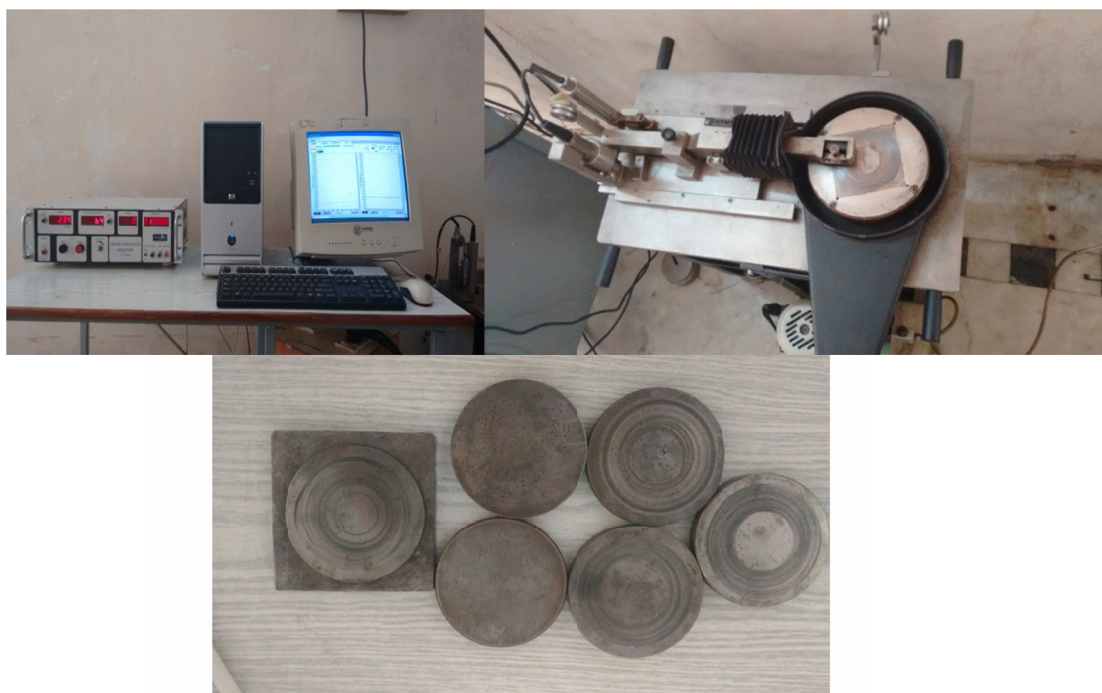
Fig. 2. Wear testing machine and Wear discs of three compositions
