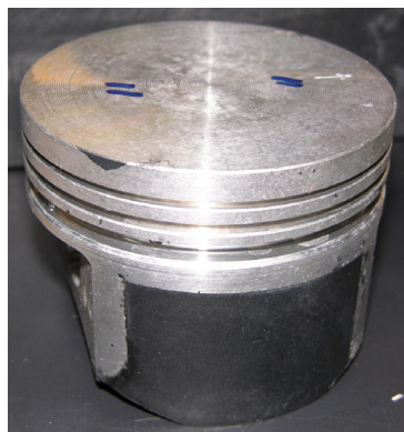
Fig. 5. The piston with a layer of nanotubes applied to the lateral surface prior to testing
