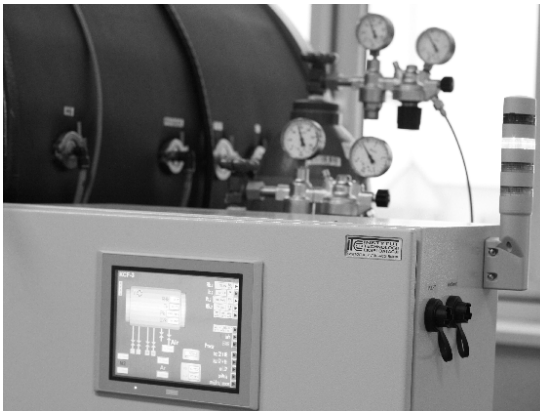
Fig. 2. Fumigation chamber: a) Realized chamber, b) The control-measurement system of the chamber – in the middle the 3-phase electricity meter, c) A view of the touch operator panel, d) Fragment of a monitoring screen for cylinders and vacuum pumps
