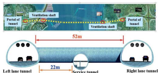
Fig. 2. Schematic diagram of the cross-section of tunnel layout
