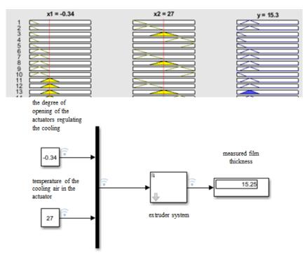
Fig. 9. Extruder operation model
