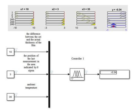
Fig. 8. Example of the operation of fuzzy controller 1 – the degree of opening of the actuators regulating the cooling
