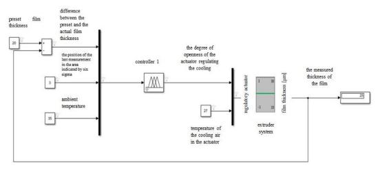
Fig. 7. The concept of simulation model to verify the operation of fuzzy control
