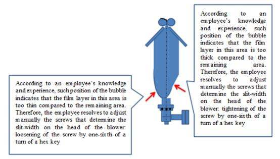
Fig. 2. Position and shape of the blown bubble
