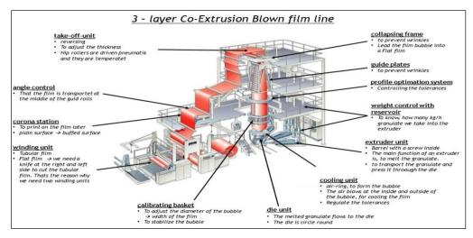
Fig. 1. A diagram of a blow extrusion machine
