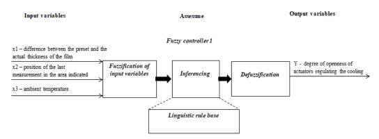
Fig. 4. Stages of the inferencing process based on fuzzy logic for the system of fuzzy controller 1
