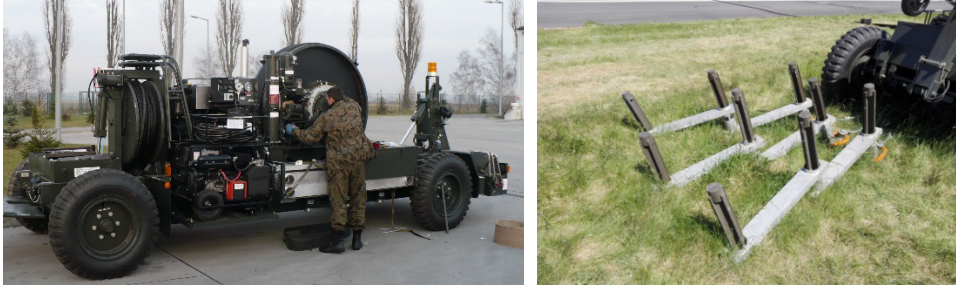
Fig. 13. Mobile devices of the BAK-12 arresting system in the transport position and anchored into the natural pavement (in the ground)
