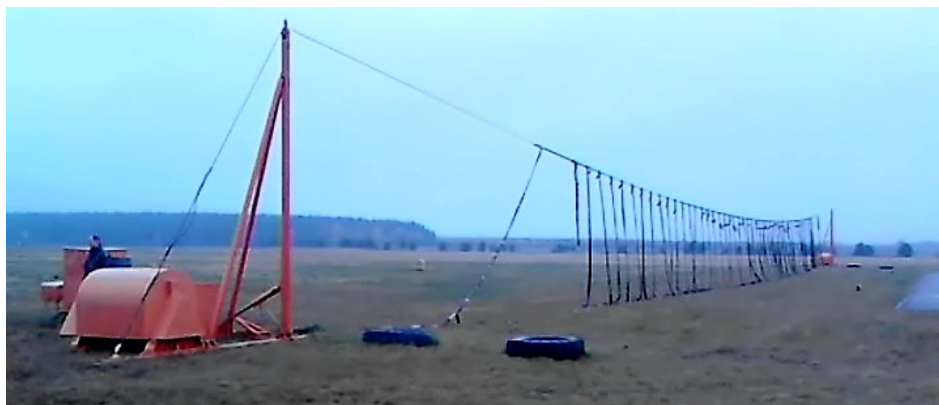
Fig. 14. ATU-2M aircraft emergency arresting system with SL-24 net ready for an arrestment – airfield in Miroslawiec in Poland
