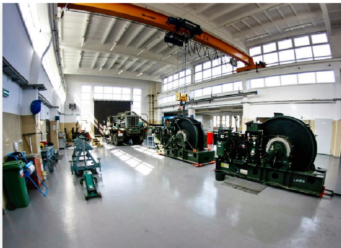
Fig. 15. Workshop hall of aircraft arresting gear systems in WTL in Toruń (Poland)
