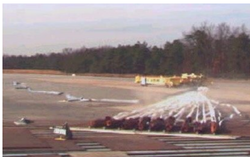
Fig. 9. Braking module of the textile brake after aircraft arrestment
