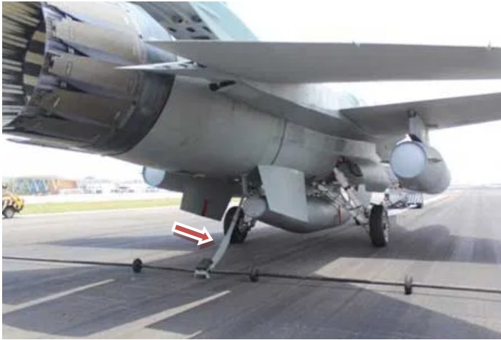
Fig. 4. Arresting gear hook in the lowered position
