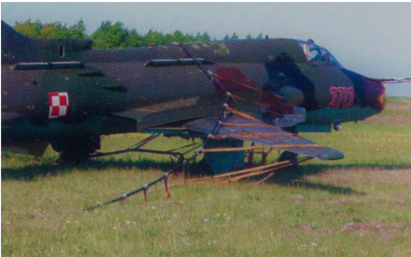
Fig. 3. Su-22 aircraft after being arrested by the ATU-2M arresting net system [Polska Zbrojna]
