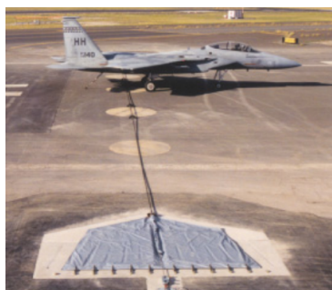
Fig. 8. Arresting cables with textile brake
