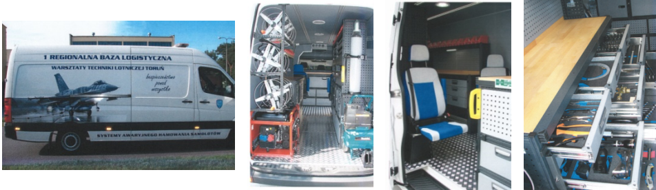
Fig. 16. Workshop truck of BAK-12 aircraft emergency arresting systems
