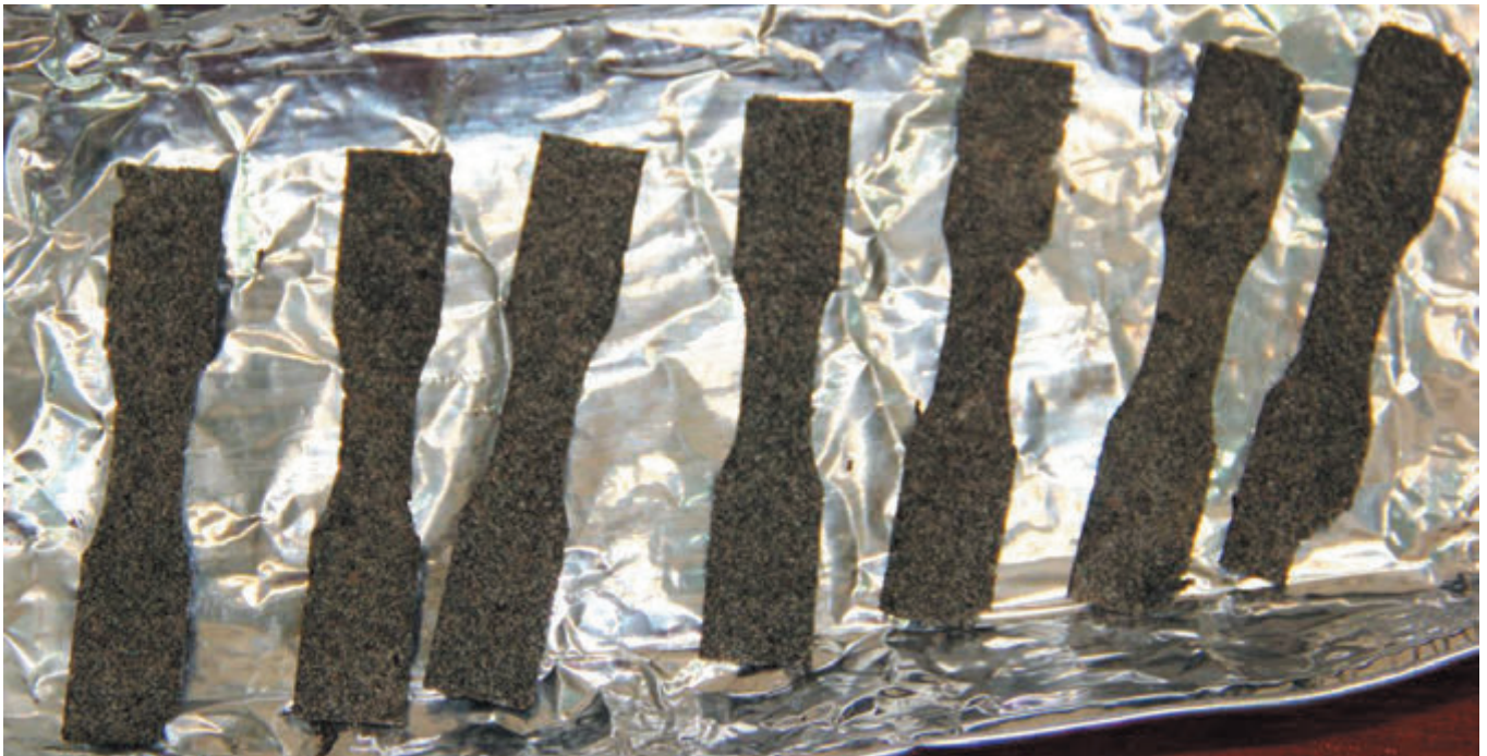
Fot. 1. Prepared for testing bitumens mass samples from Żelazny Most (on the surface glued monolayer of flotation sludge is visible)
