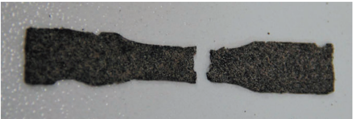
Fot. 2. An example of bituminous mass sample after tenacity examination
