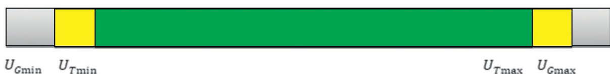
Fig. 2. Narrowed voltage range of the generator
