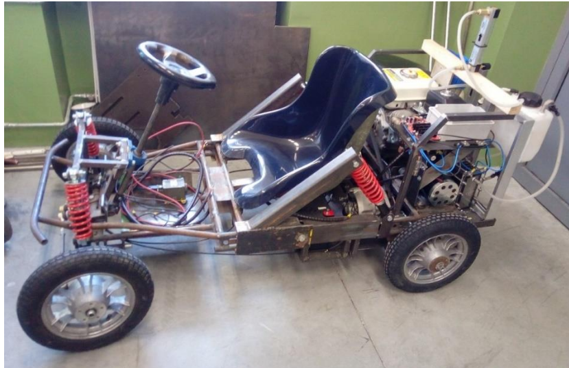
Figure 1. View of the test vehicle without car body
