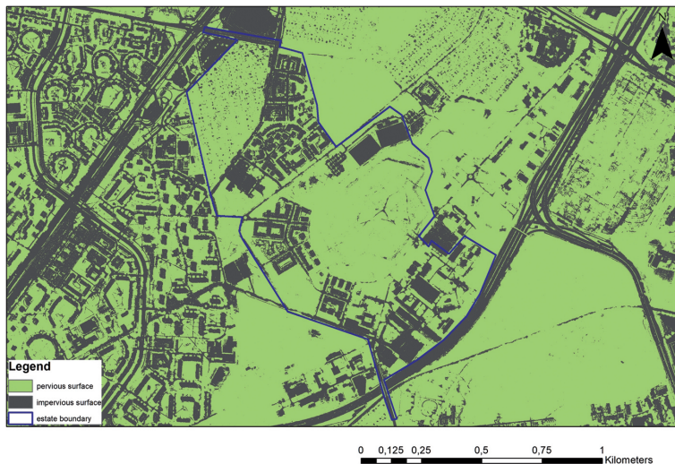
Fig. 4. Results of the classification (mapping) of impervious surfaces with the SVM method [source: own elaboration in ArcGIS 2.9]
