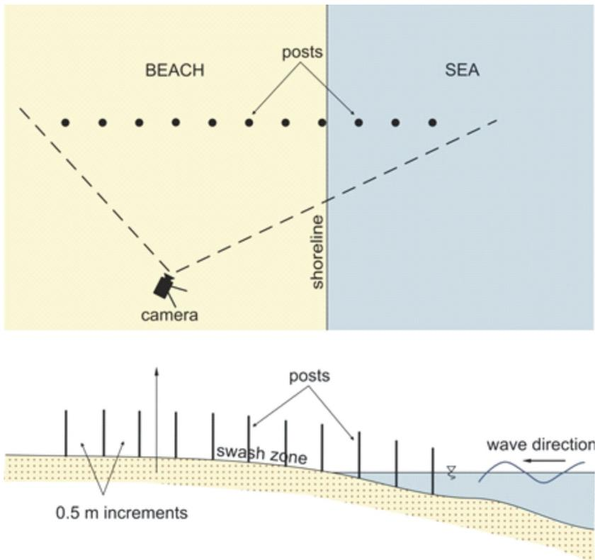
Fig. 4. Setup for beach run-up height recordings at Lubiadowo in 2016
