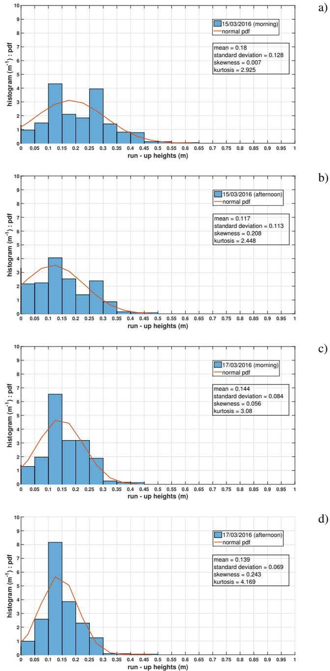
**Fig. 6.** Histograms and empirical probability density functions of wave run-up for a) Mar. 15, 2016, morning; b) Mar. 15, 2016, afternoon; c) Mar. 17, 2016, morning; d) Mar. 17, 2016, afternoon
