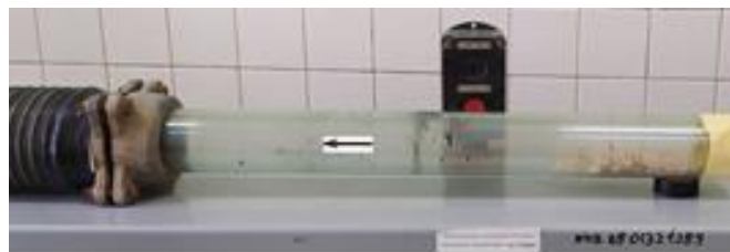
Figure 3. Laboratory test stand (fragment) for research pickup velocity air flow of CW settled in a horizontal duct
