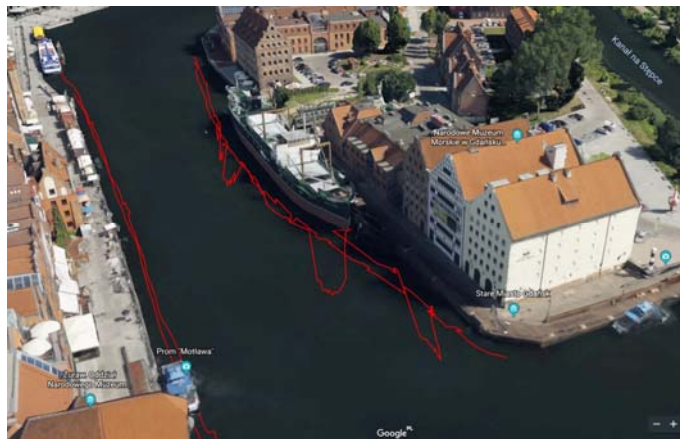
Figure 3. Hydrographic vessel's trajectory in highly congested, narrow canal area (Gdansk – Motlawa)
