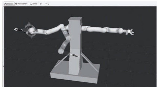
Fig. 7. Motion planning for Bilateral KUKA LWR Robot Platform in Moveit! using interactive marker
