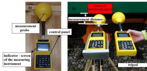
Fig. 3. Electromagnetic field meter EFA-300 with attached measuring probe, a) general view of instrument, b) instruments on measuring stand on railroad track
