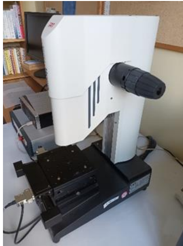
Fig. 2. MicroSpy® Profile profilometer by the FRT the art of metrology™. Source: [own source].
