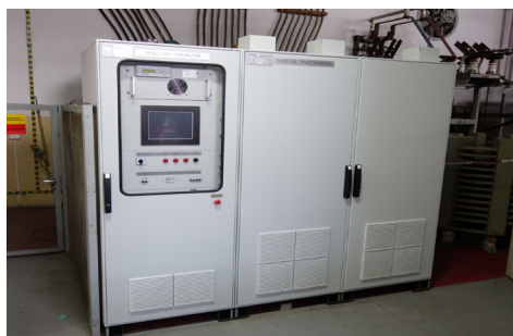
Fig. 2. a) DC / DC-350 converter in a short-circuit laboratory [9]; b) View of the inverter control panel - sample data sent by the BMS (Battery Management System) to the inverter [13]
