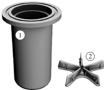
Fig. 4. Pit furnace retort (1) and base for its installation at the bottom of the furnace chamber (2) [5]; material: GX40CrNiSi25-20, GX40NiCrSi35-17 or GX40NiCrSiNb38-19 or steel of similar chemical composition
