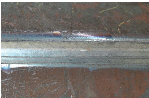
Fig. 2. A view of the face of the weld made by the 121 method in a flat position – PA
