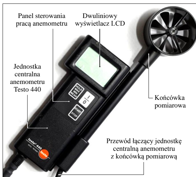
Rys. 4. Widok ogólny anemometru Testo 440 [20] Fig. 4. General view of the Testo 440 anemometer [20]
