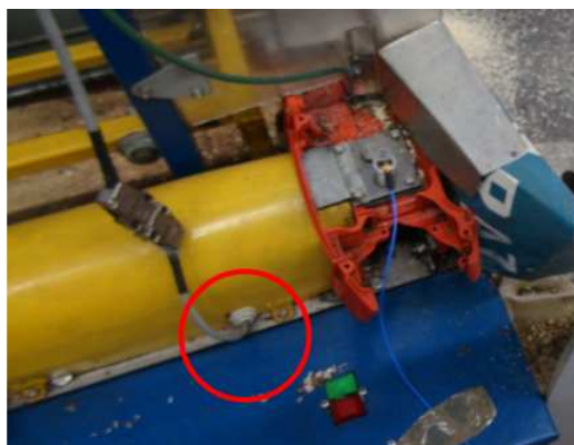
Fig. 1. View of mounted torque transducer and laser vibrometer
