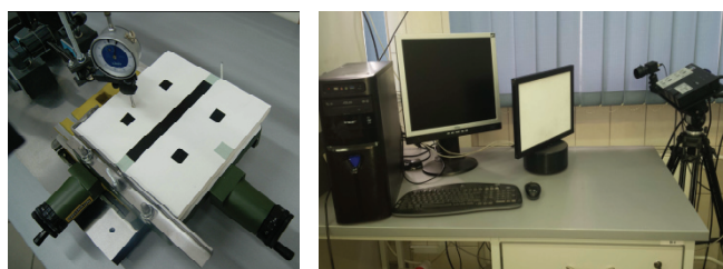
Fig. 5. Measuring equipment for measurement of the thickness of paint layers, dial thickness gauge (on the left) and 3D scanner (on the right)
