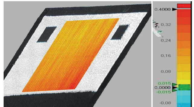
Fig. 10. Visual image example of the surface structure of the tested coating obtained by means of 3D scanner
