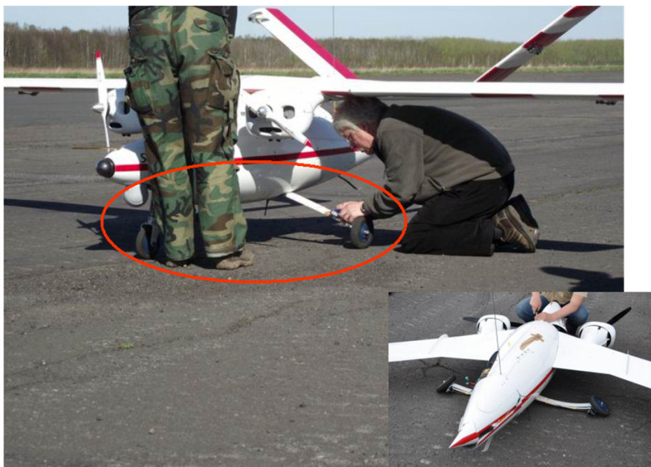
Fig. 18. Landing gear of SAMONIT 1
