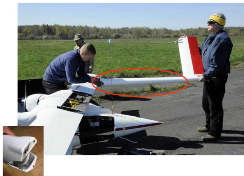
Fig. 16. Tail beam of SAMONIT 1
