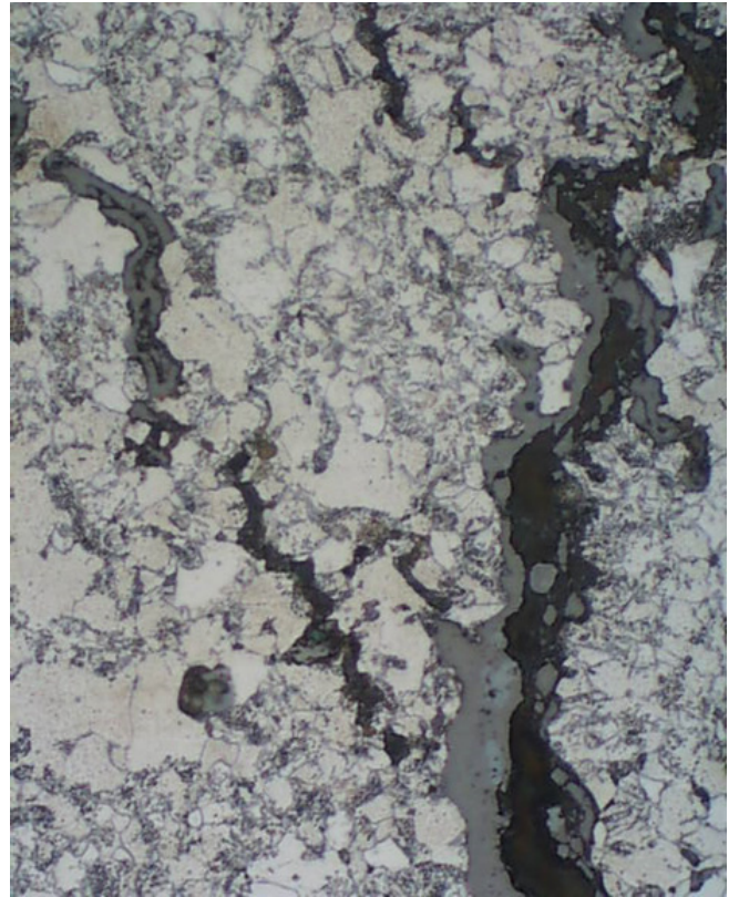
Fig. 8. HAZ – the bainite type of a structure. The disintegration of the primary structure, grids of intercrystalline macro and microcracks, and the chains of creeping micropores on the grain boundaries. Zoom 500×
