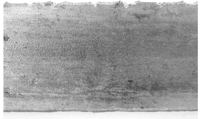
Fig. 10. Example view of part of flat thick 5 mm made by cold rolling from \phi 30 mm Al continuous ingot in initial state
