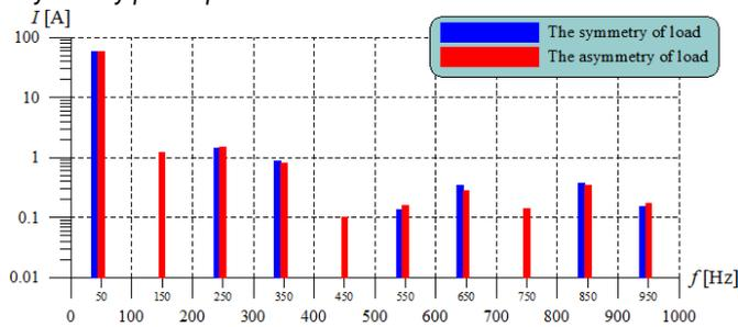
Fig. 9. The frequency analysis of generator current with symmetry and asymmetry point operation – the result of simulation.
