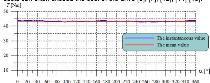
Fig. 1. The waveform of electromagnetic torque for generator loaded symmetrically.
