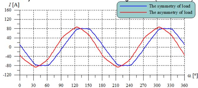
Fig. 8. The waveforms of generator current with symmetry and asymmetry point operation – the result of simulation.
