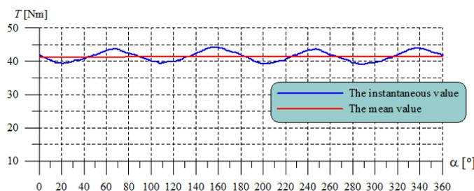
Fig. 2. The waveform of electromagnetic torque for generator loaded asymmetrically (the current in one phase  $I = 0,75 I_n$ ).
