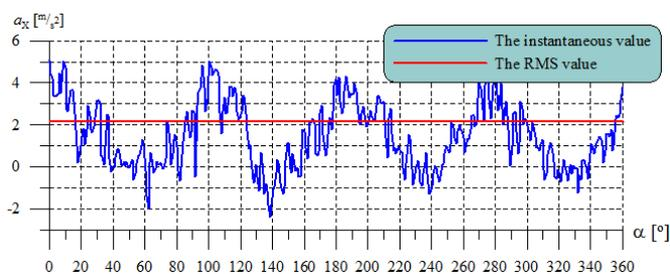
Fig. 6. The waveform of vibration acceleration for generator loaded asymmetrically (the break in one phase).
