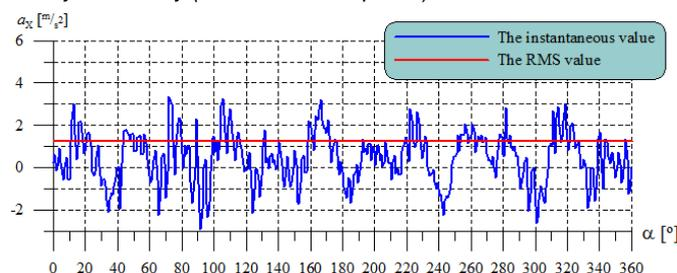
Fig. 4. The waveform of vibration acceleration for generator loaded symmetrically.
