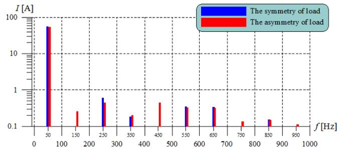
Fig. 11. The frequency analysis of generator current with symmetry and asymmetry point operation – the result of laboratory tests.
