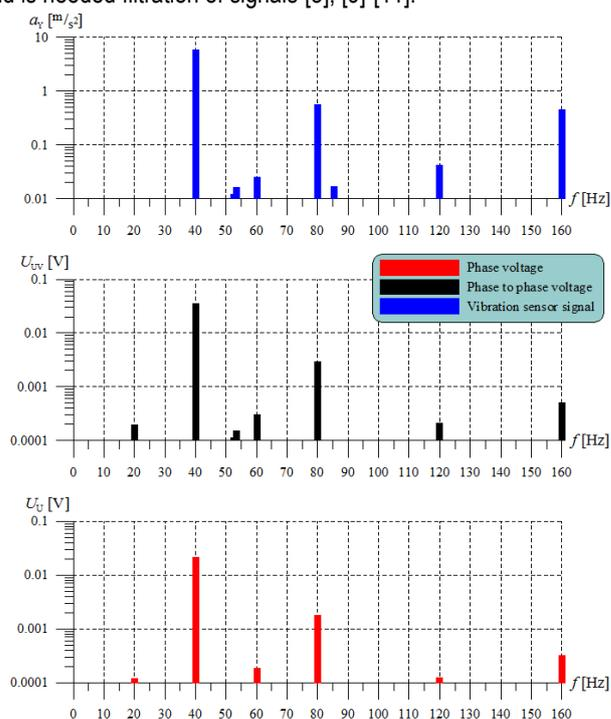
Fig. 7. The frequency analysis of signals: own and vibration sensor –static tests on the vibration table.
