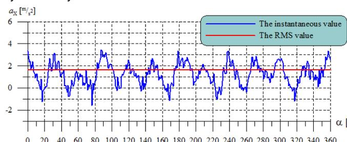
Fig. 5. The waveform of vibration acceleration for generator loaded asymmetrically (the current in one phase  $I = 0,75 I_n$ ).
