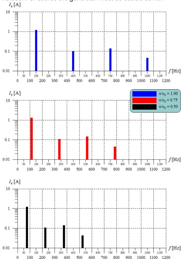
**Fig. 13.** The frequency analysis of generator current for asymmetry of point operation for several rotational speeds.
