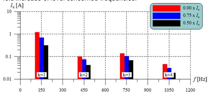
Fig. 12. The frequency analysis of generator current for several asymmetries of point operation.
