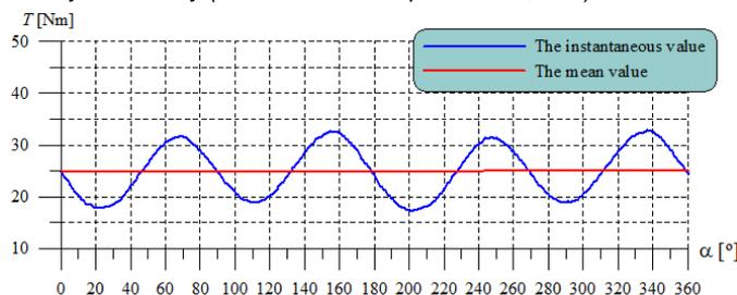
Fig. 3. The waveform of electromagnetic torque for generator loaded asymmetrically (the break in one phase).
