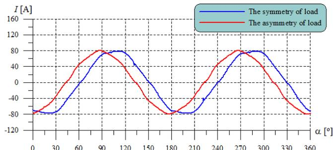
Fig. 10. The waveforms of generator current with symmetry and asymmetry point operation – the result of laboratory tests.
